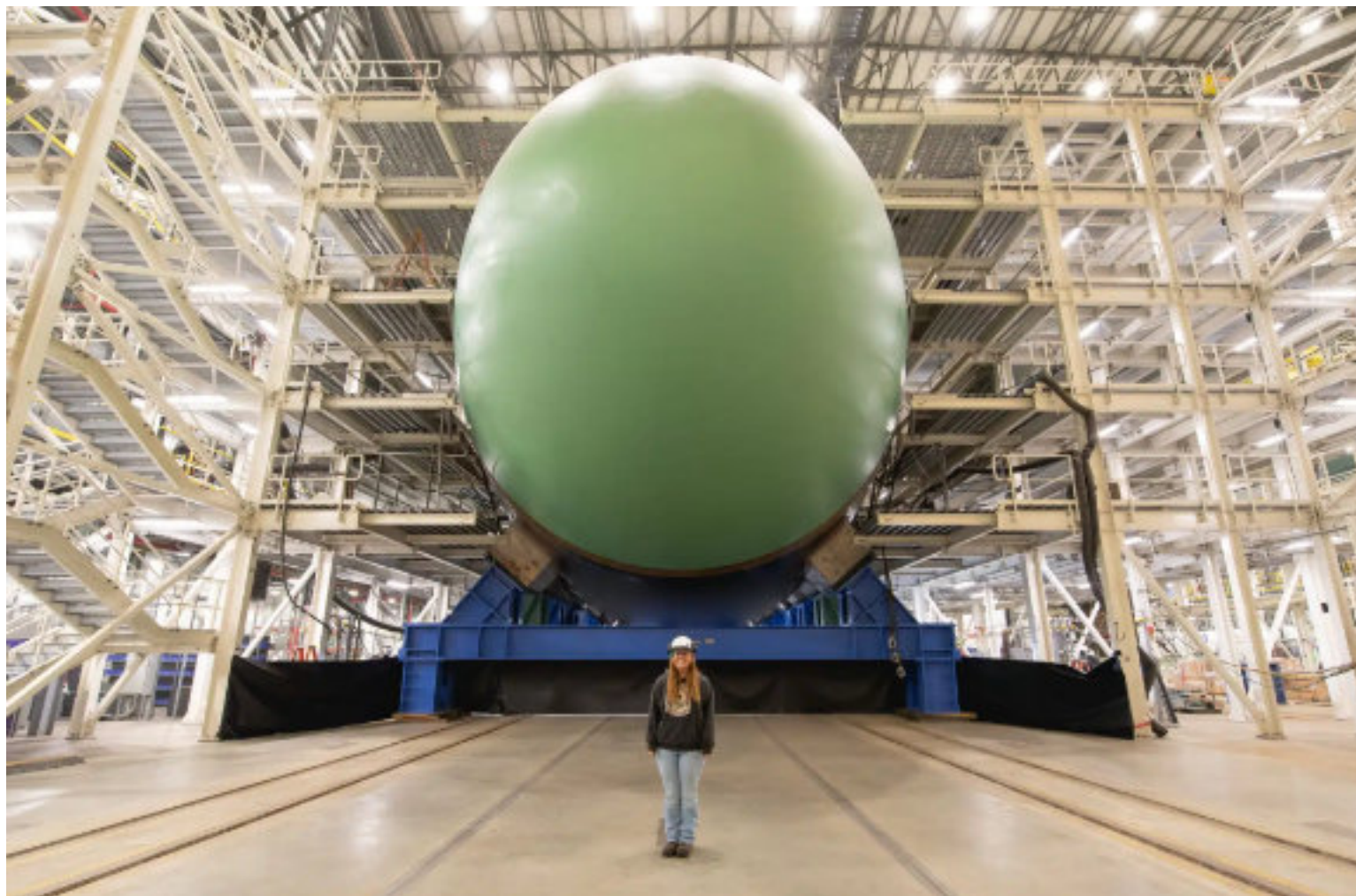
The completed bow section of the future USS District of Columbia, pictured indoors for the first time. Photo from Ashley Cowan's LinkedIn.
