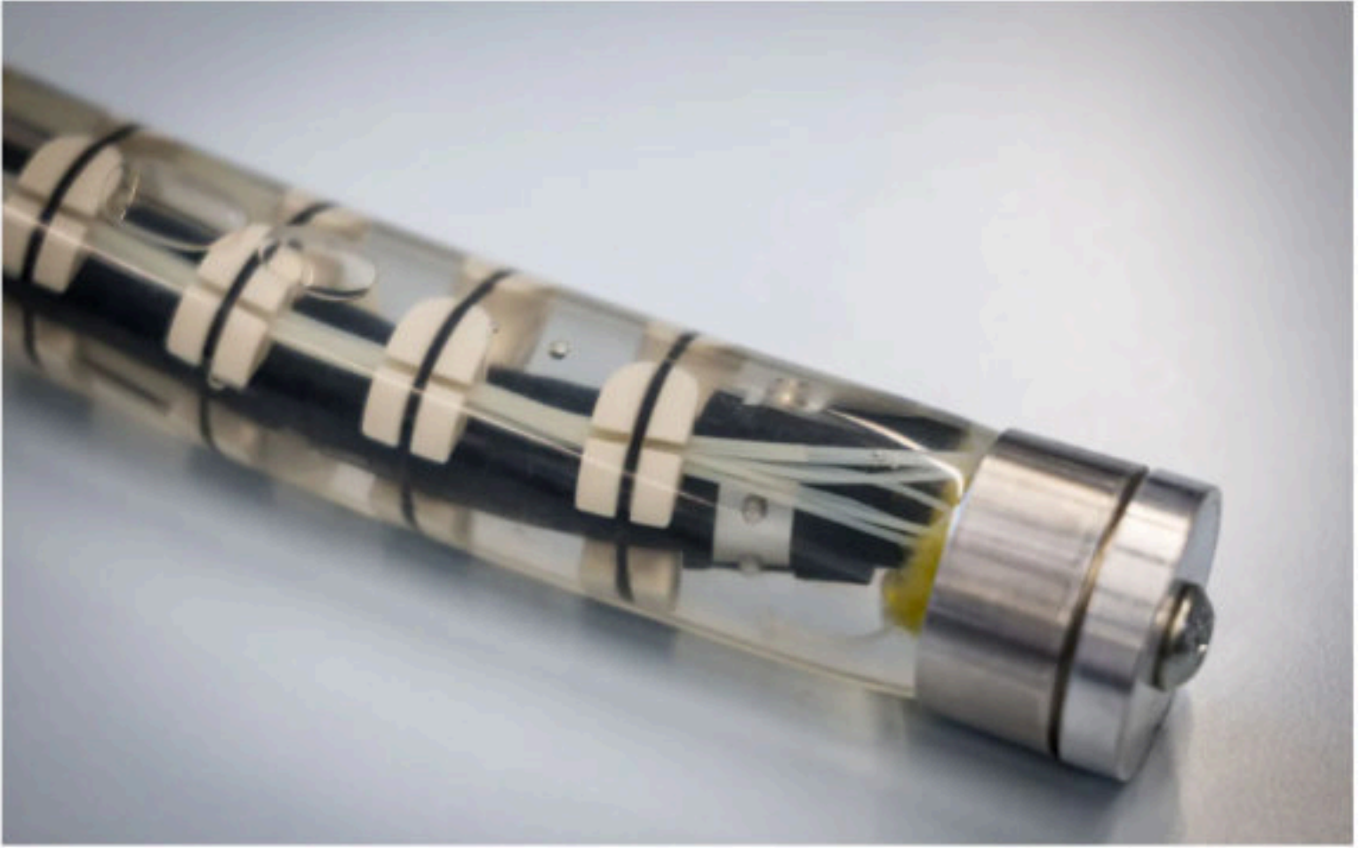
Optic11's towed array sensor cable can be deployed from any warship or civilian vessel Credit: Dutch Military Defence/Sjoerd Hilckmann
