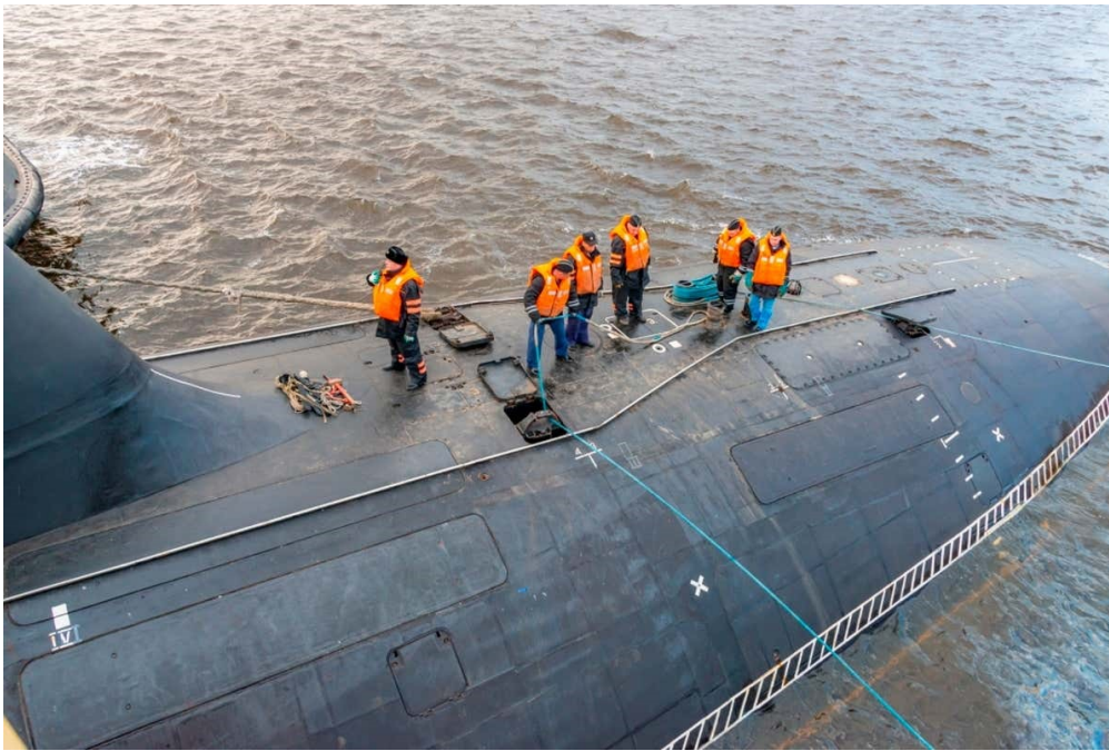
Crew on the hull of Kazan while in harbor. Note the hatches for torpedo loading (on the left of the picture) and torpedo launch (on the right)
