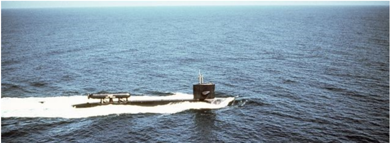
USS Parche was a Cold War era attack submarine modified to conduct spy missions underwater. Parche featured a number of unique modifications, including ski legs that allowed it to rest on the seabed. Today the USS Jimmy Carter conducts similar missions, though without the tiny submarine legs.
