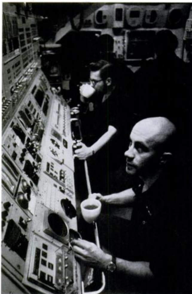
CONTROL CENTER. Heart of George Washington —equivalent to the bridge of a surface warship—is a complex, computer-crammed area from which sailors steer the ship. With a pair of "joy sticks," like the one at top, they angle her up and down and turn her.
