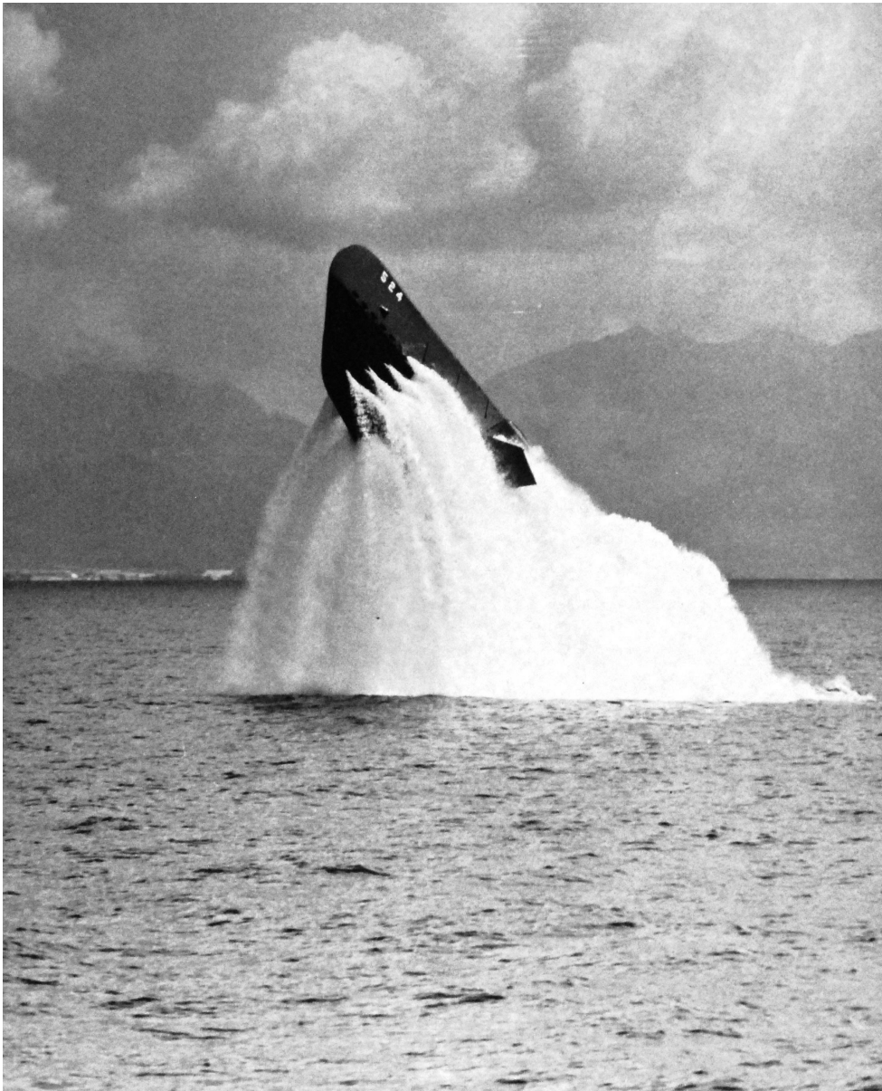
Tench class USS Pickerel (SS-524) performing an emergency surface test from a depth of 150 feet with a 48° up-angle off the coast of Oahu, Hawaii, 1 March 1952.
