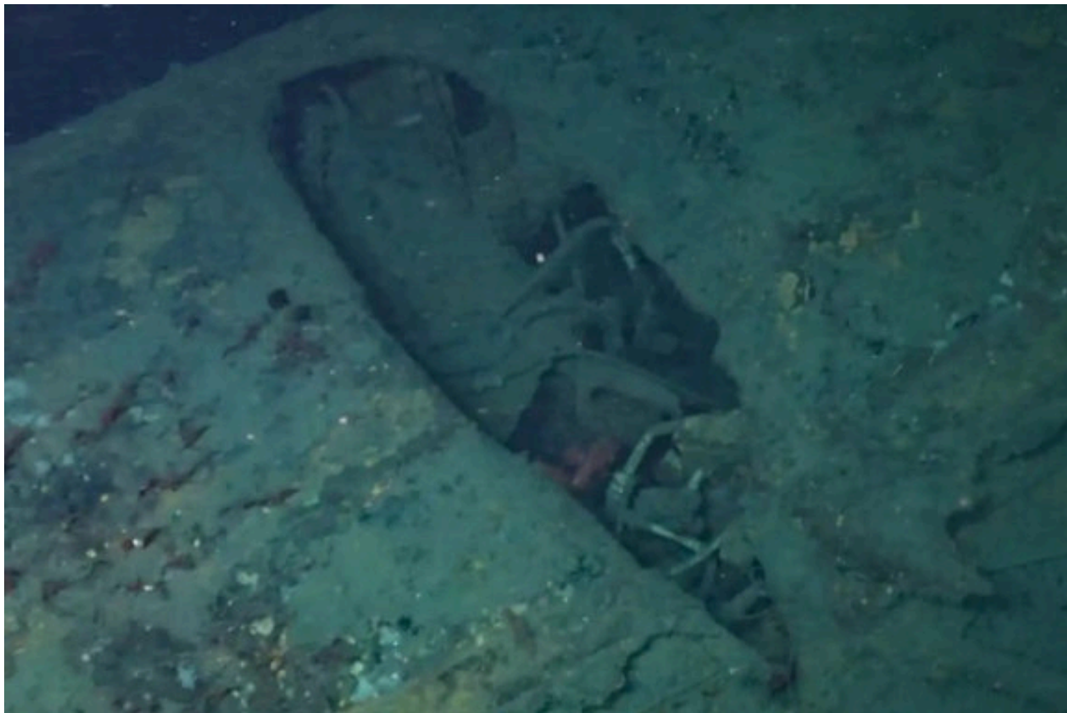
The detailed photogrammetric reconstruction of the USS F-1 showing the conning tower and collision damage that caused the sub to sink (Image: Zoe Daheron/Woods Hole Oceanographic Institution)
