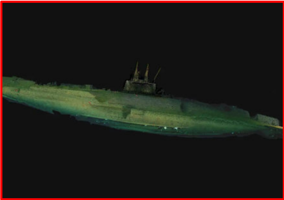
Photogrammetric reconstruction of the submarine USS F-1 (Image: Zoe Daheron/Woods Hole Oceanographic Institution)
